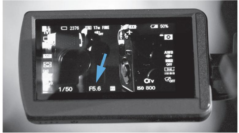
■ **Figure 10-22** Most film and video lenses designed for film production have engraved aperture f-stops (*left*); however, some lower-end camcorders will only show f-stops on the LCD viewscreen (*right*).
