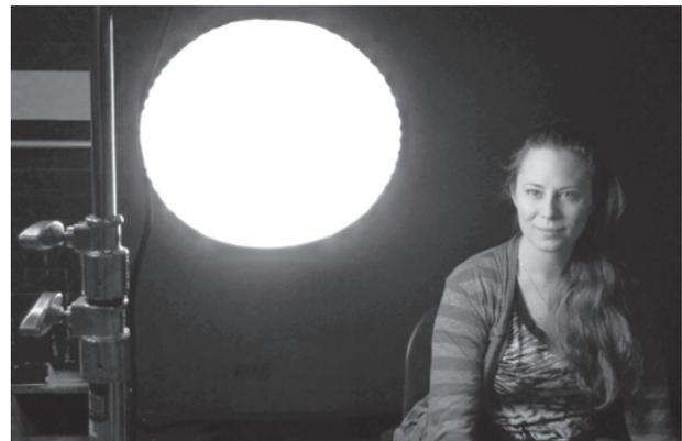
■ **Figure 13-50** "Chinese lantern" globes provide a source of soft light, especially for close-ups on faces.
