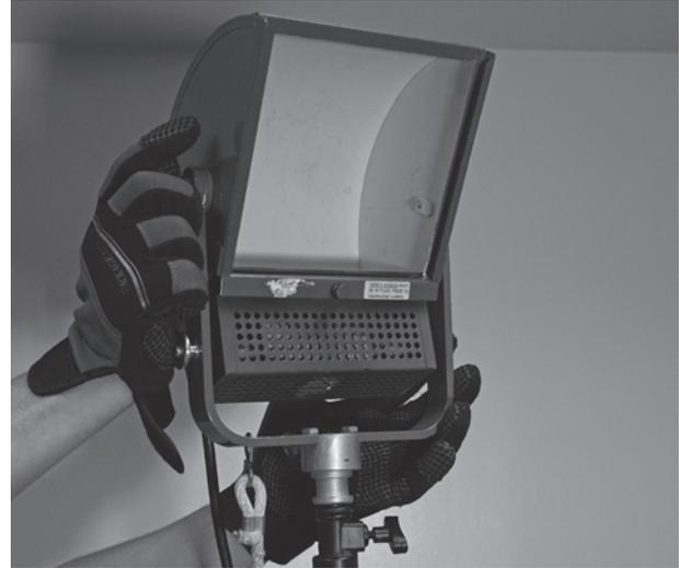
■ **Figure 13-49** Many soft lights illuminate by bouncing light off some form of diffusing reflector. This Mole-Richardson 750-watt baby-soft has a matte white shell reflecting the light from a recessed lamp.
