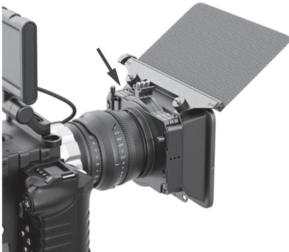
■ **Figure 13-37** Matte boxes sit in front of a camera lens and block unwanted light from hitting the lens. They can also have filter holders for rectangular glass or plastic filters. This matte box accommodates three filters (arrow).
