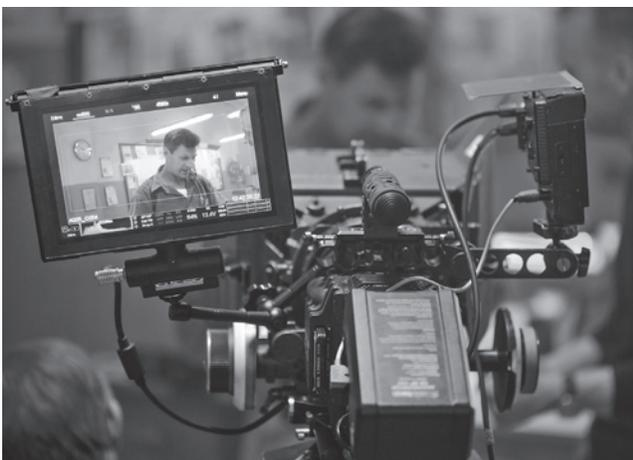
■ **Figure 12-16** High-resolution, portable field monitors are an indispensable tool for narrative filmmakers. In addition to simply monitoring your image, they often offer a variety of image evaluation scopes and some can even serve as a secondary recording device.
