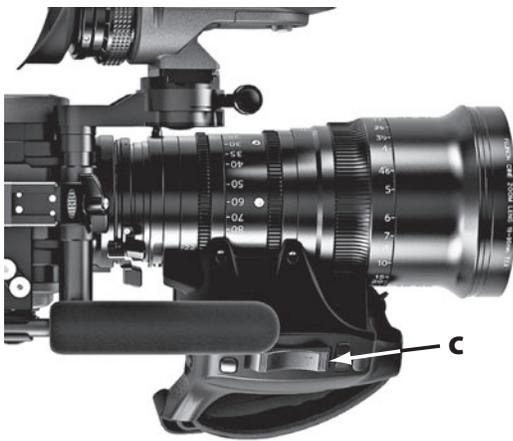
■ **Figure 10-6** A zoom lens changes focal length by shifting the position of the internal optical center elements (a) by adjusting the zoom ring (b) (*top*). Some cameras have a servo zoom motor controlled by a rocker switch (c) that lets you glide from one focal length to another (*bottom*).
