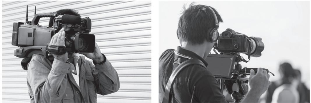
■ **Figure 9-2** Some camera bodies are designed for handheld work, like shoulder-mount camcorders (*left*), while other camera body shapes require some form of camera support, like DSLRs which are awkward to hold and benefit from a tripod (*right*) or some form of camera rig.
