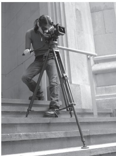
■ **Figure 11-9** The individually extendable legs of a tripod make it possible to get stable support on uneven surfaces, such as a staircase.
