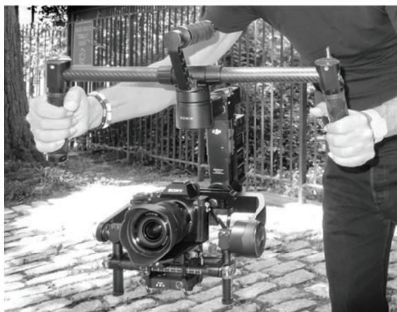
■ **Figure 11-17** The emergence of small video and DSLR cameras has prompted the creation of lighter, cheaper stabilizing systems, like this Glidecam (*left*) being used for a moving shot. Gimbal stabilizers use computer controlled motors, like this DJI Ronin—M (*right*).
