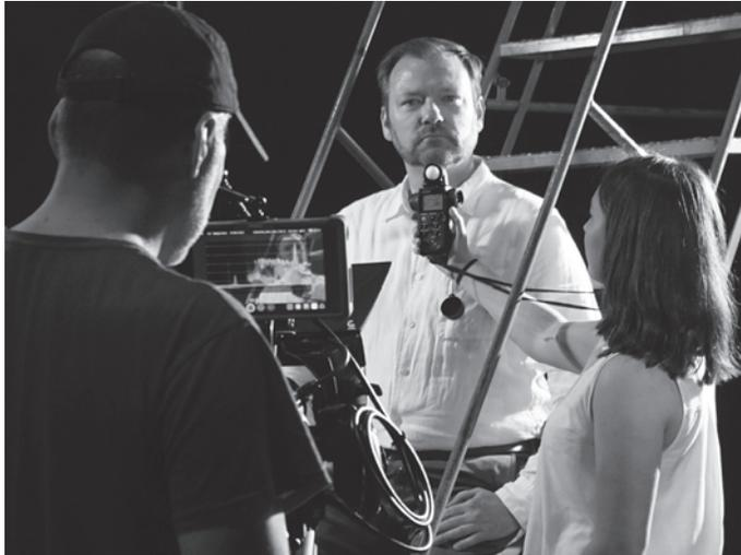
■ **Figure 14-15** An incident light meter should be positioned at the subject with the photosphere pointing toward the lens of the camera.
