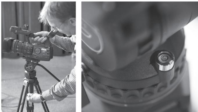
■ **Figure 11-8** A camera operator adjusts the level of the tripod head by loosening the ball and socket mount (*left*) and using the bubble leveler at the base of the head (*right*).
