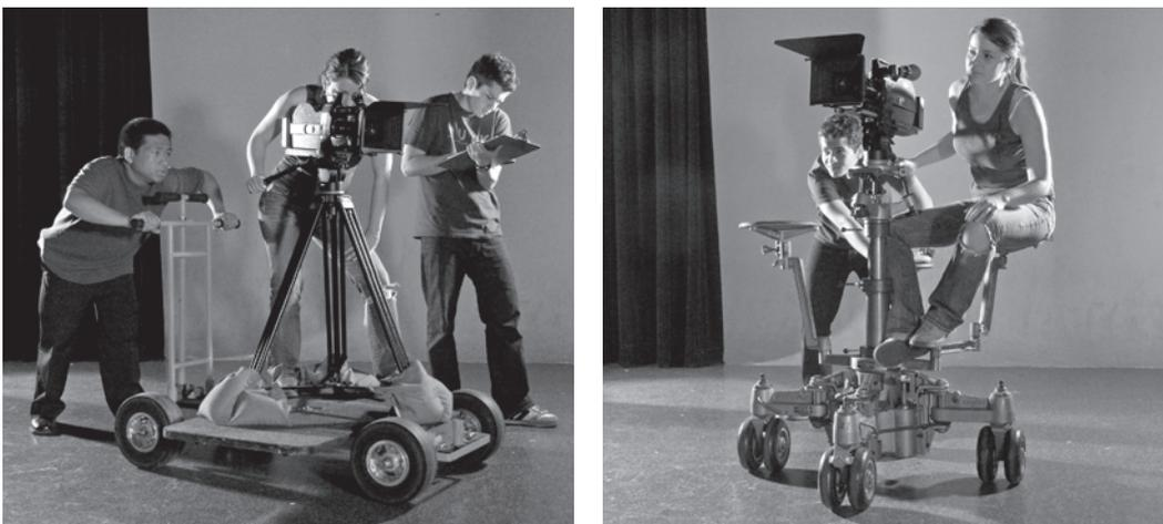
■ **Figure 11-12** A doorway dolly (*left*). Inflatable wheels allow for a smooth transit and do not require tracks. A spider dolly, capable of crablike lateral moves (*right*).
