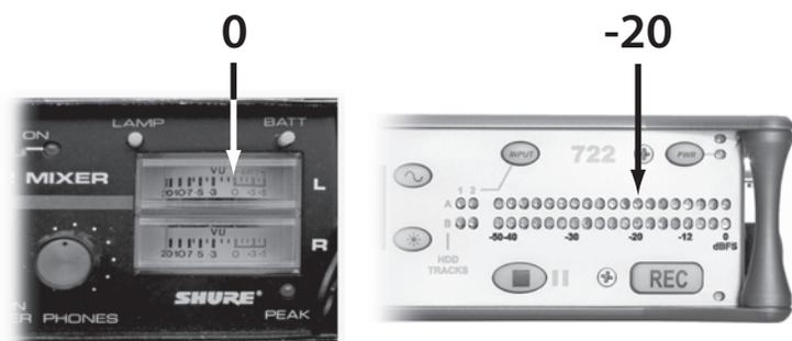
■ **Figure 16-5** A 1kHz reference tone is used to calibrate the output of the mic mixer with the input of the recorder (or camcorder). The mixer’s VU meter reads the reference tone at 0dB (*left*), whereas the recorder’s peak meter should be set to register the tone at  $-20\text{dB}$  (*right*).
