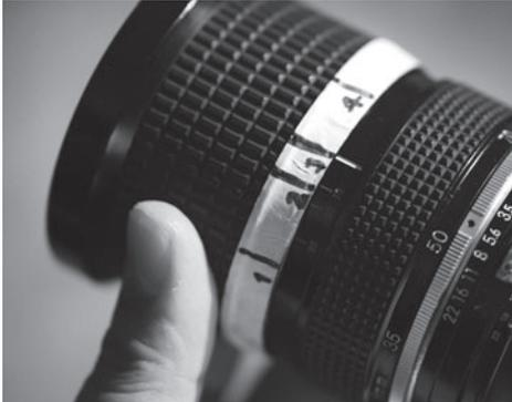
■ **Figure 10-19** A follow focus device (*top*) allows you to mark predetermined focus points for easy focus pulling. If you don't have this device, using paper tape on the barrel of a lens (*bottom*) can accomplish the same thing.
