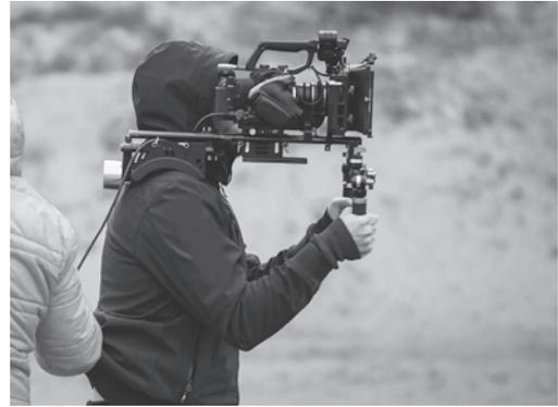
■ **Figure 11-3** With small digital cameras and DSLRs, camera operators often prefer to use a shoulder-mount rig to improve control for handheld shots.
