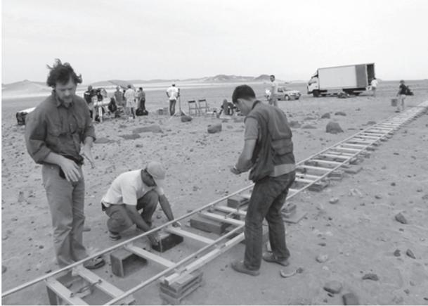
■ **Figure 11-13** Dollies that use tracks can create extremely smooth moving shots, even over rough terrain, but their setup is a time- and labor-intensive endeavor.
