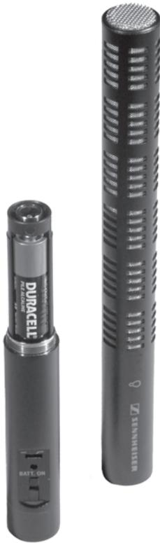
**Figure 15-25** Condenser microphones, like the Sennheiser shotgun pictured, need a battery to provide the power necessary to charge the capacitor.
