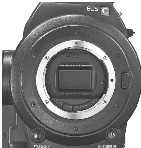
■ **Figure 9-16** You will find the camera image sensor, in this case a single CMOS sensor, directly behind the lens mount.
