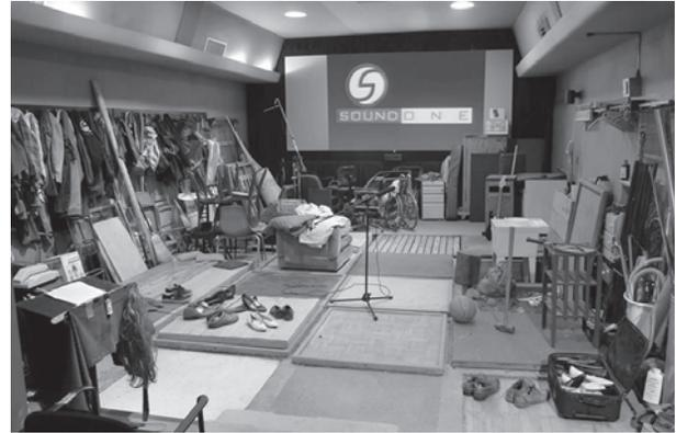
■ **Figure 22-13** Professional foley rooms are sound studios designed to record postsynchronous sound effects while the foley artist watches the scene projected. As you can see here, they are outfitted with a wide array of objects that can make a variety of noises.
