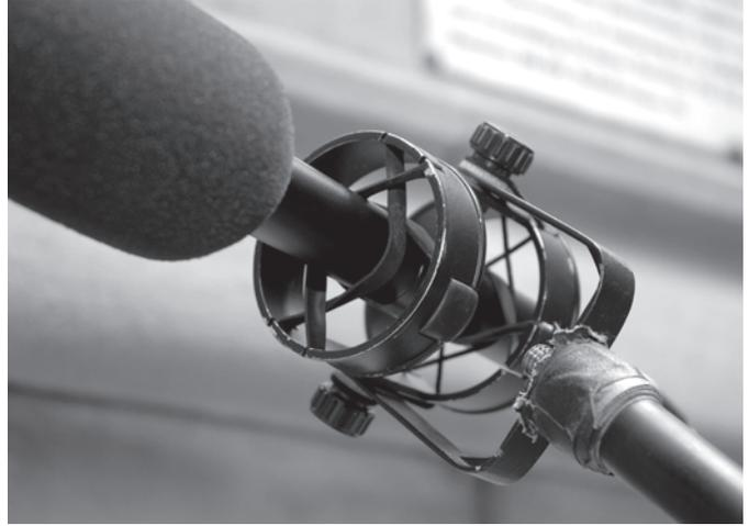
■ **Figure 16-10** A shock mount keeps the microphone secured and prevents it from picking up vibrations caused by moving the boom pole.
