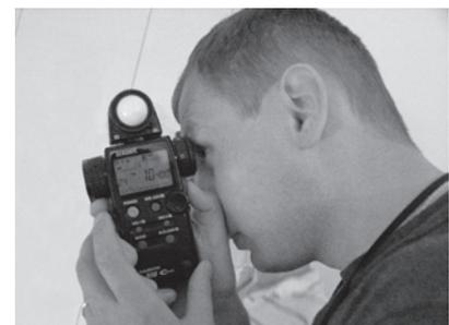
■ **Figure 14-14** The most common handheld meter for film production is the incident meter, like this affordable Sekonic L-308DC which is designed for use with video cameras (left). A spot meter is a reflected light meter and can be useful for measuring exposure values from a distance or for objects that emit light. Shown here is a Sekonic combination incident/spot meter (right).
