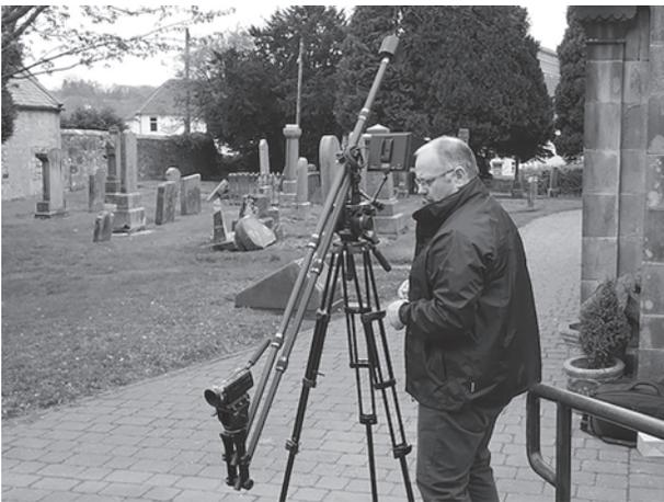
■ **Figure 11-15** Jib arms are extremely versatile camera supports. This compact jib arm designed for small digital cameras will allow an operator a range of camera moves like pan and tilt, boom up and down, swing in an arc, or suspend the camera directly over a subject.
