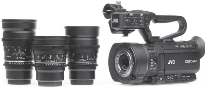
■ **Figure 9-5** This JVC digital camera has a lens mount for interchangeable lenses that include prime lenses or zoom lenses.
