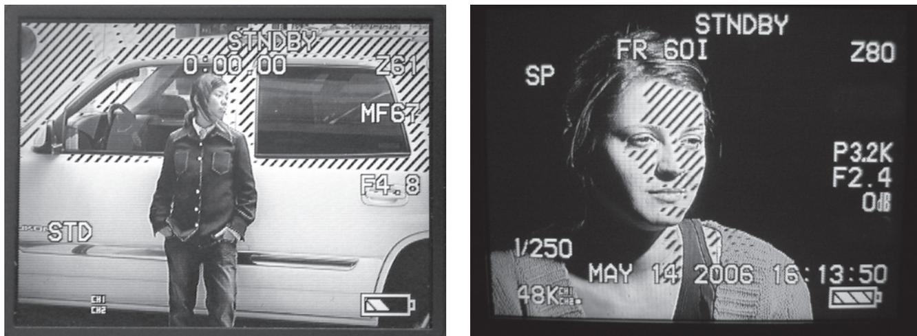
■ **Figure 12-15** The zebra stripe function is useful to control overexposure in our shots. Zebras are usually calibrated to display overexposures in white areas (100%) (*left*); a lesser used zebra pre-set is for "correct" exposure on Caucasian face tones (70%) (*right*).
