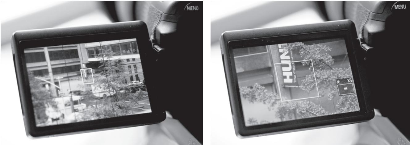
■ **Figure 10-17** To aid with critical focus, many video cameras offer a focus assist function, which magnifies a portion of the scene (*right*).
