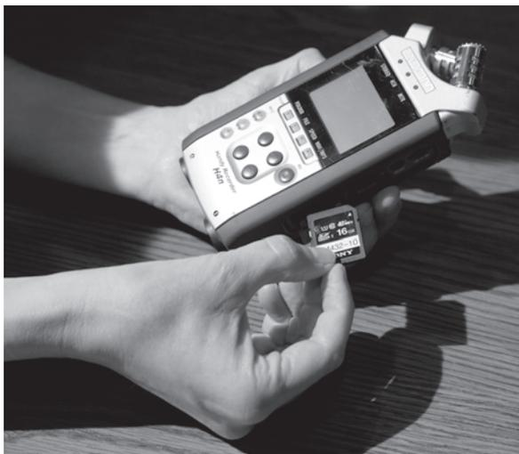
■ **Figure 15-19** With no moving parts and consuming very little power, SD (pictured) and CF memory cards allow for small, yet sturdy digital recorders.
