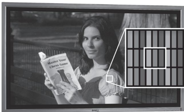
■ **Figure 8-15** Just like camera sensors, color flat-screen displays (LCD or plasma) are made up of millions of pixels. Each individual pixel contains red, green, and blue subpixels (*outlined*). See the color insert.
