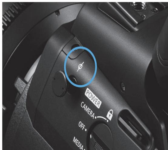
■ **Figure 10-2** The image plane symbol marking on Canon C-100 (circled).
