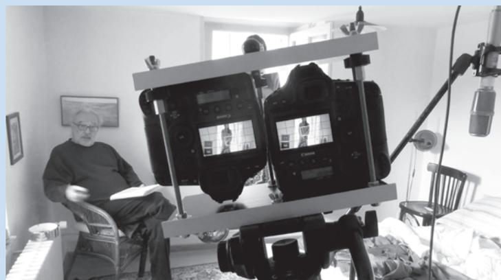
■ **Figure 9-37** The future of 3D filmmaking beyond the blockbuster is still in question despite the marketing of 3D camcorders like this Sony PMW-TD 300 3D (*left*) and the explorations of prominent filmmakers like Jean Luc Godard, shown here on the set of *Adieu Au Langage* with a double DSLR 3D rig (*right*).
