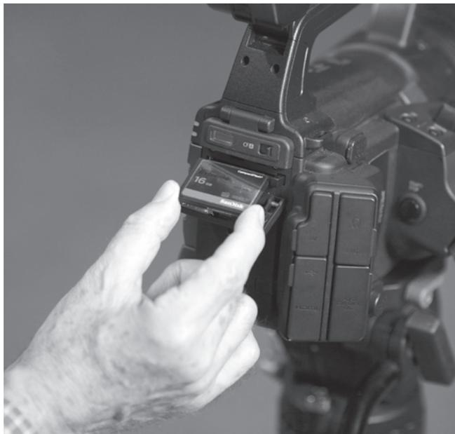
■ **Figure 9-9** File-based recording on solid-state memory cards offers many advantages and is now the standard. The Canon XF300, pictured here, has two CF card slots to allow for longer, continuous recording.
