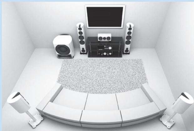
■ **Figure 23-28** Surround sound 5.1 is an alternative to mono or stereo mixing and is required for DCPs. It involves mapping six audio channels to six speakers for playback. Pictured is a typical surround sound 5.1 speaker setup: three front, two back, and a sub-woofer.
