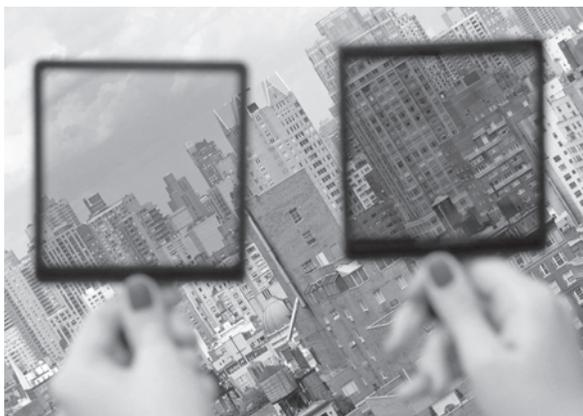
■ **Figure 13-38** Neutral density filters cut the amount of light entering the lens without changing its color. ND 0.3 (left) reduces light by 1 stop and ND 0.6 (right) cuts the light by 2 stops. These are 3 × 3 filters that fit into a matte box filter holder.
