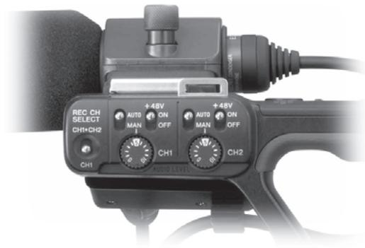
■ **Figure 16-6** The auto gain control found on many video cameras should be turned off to have precise manual control over the audio recording levels.
