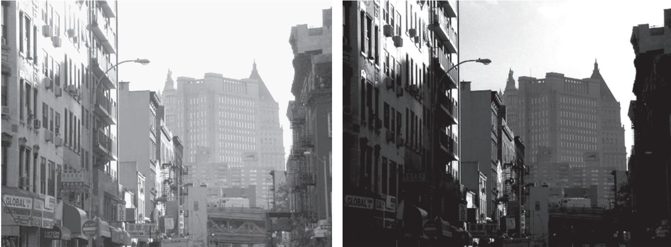
■ **Figure 14-3** When the contrast range of a scene exceeds the dynamic range of the camera, exposures must be carefully chosen. The image on the *left* exposes the street level signs correctly, but the brighter areas (like the sky and the center building) become overexposed. The image on the *right* exposes the center building correctly, which plunges the street level into dark shadows with little detail.
