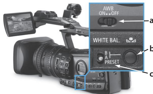
**Figure 9-29** All video cameras have a way to balance the image sensor to a variety of color temperatures. For manual white balancing you must first switch off the auto white balance function (a). A user can manually set color temperature balance for each scene (b) or recall daylight and tungsten presets (c).
