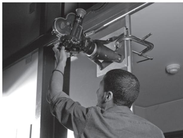
■ **Figure 11-11** A high-hat allows the camera to be placed close to the ground or attached to other surfaces with the use of clamps, as pictured.
