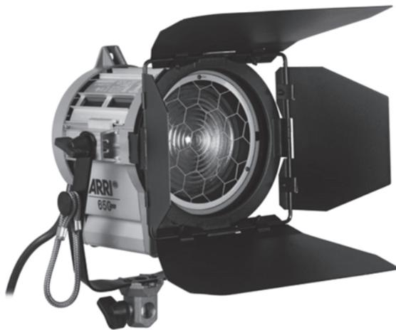
■ **Figure 13-56** Foldable barndoors like these are mounted on the front of most movie lights and help control where the unit's light falls.
