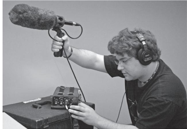
■ **Figure 16-12** Recording sound in close quarters can make handling a boom cumbersome; for these situations, a pistol grip is more convenient.
