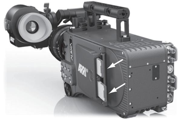
■ **Figure 19-7** The Arri Alexa camera saves uncompressed 2K–4K video to high-capacity hard drives and *simultaneously* records NLE-ready Apple Pro Res proxies to onboard memory cards (arrows) for instant off-line editing.
