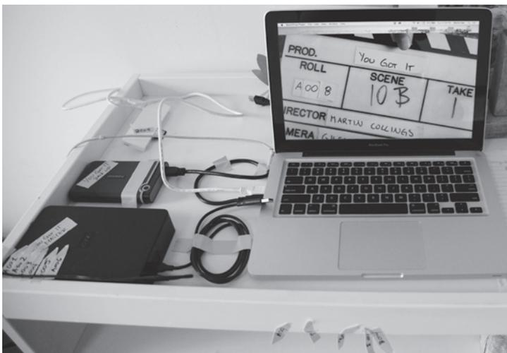
■ **Figure 17-17** A typical data management/footage backup station with a card reader, two backup hard drives, a portable computer, and tape for labels.
