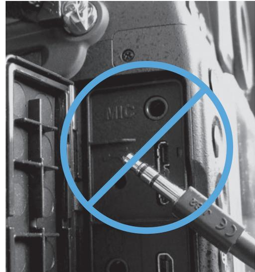
■ **Figure 15-17** DSLR cameras (pictured) and consumer grade audio equipment commonly use a mini plug for connecting microphones. This connection is flimsy and prone to interference and should be avoided if possible.
