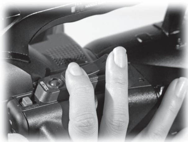
■ **Figure 9-6** A servo zoom rocker-switch allows you to easily glide through the range of focal lengths available on the lens while shooting handheld.
