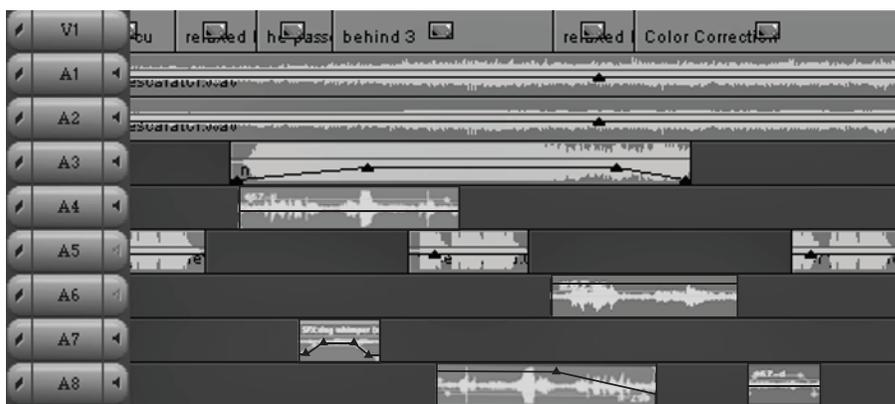
■ **Figure 23-1** The timeline for this project has eight tracks of audio—one stereo pair and six mono tracks. NLE systems can layer upward of 99 tracks of audio.
