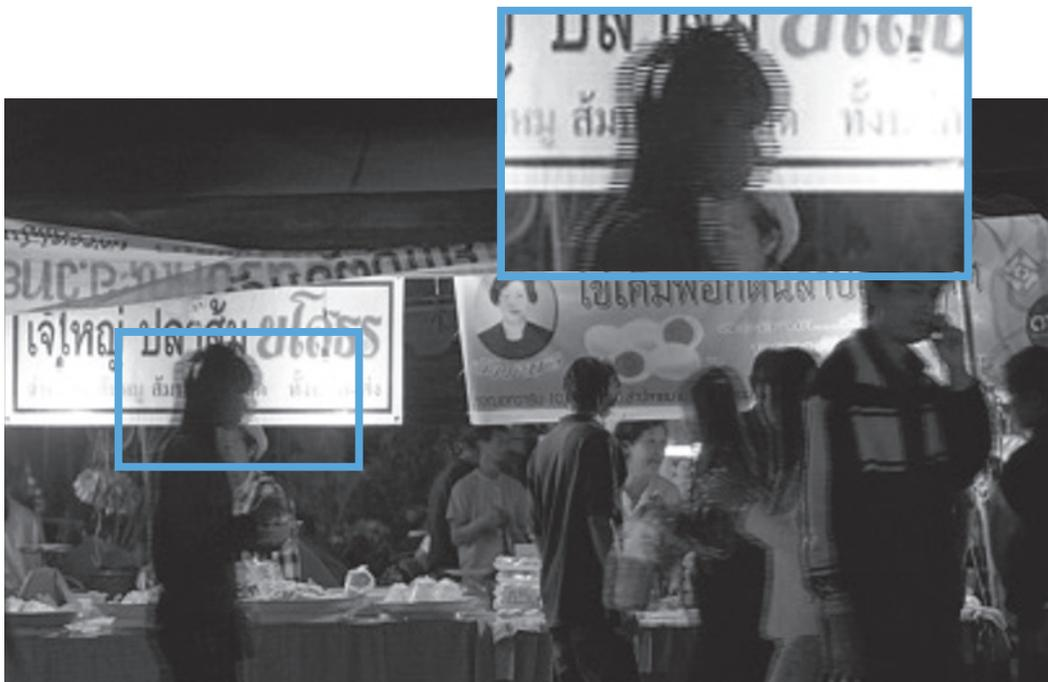
■ **Figure 8-8** When interlaced video is shown on progressing displays, a “combing” artifact occurs at the edges of moving objects caused by the displaced scan lines (notice that the stationary objects do not show any combing)
