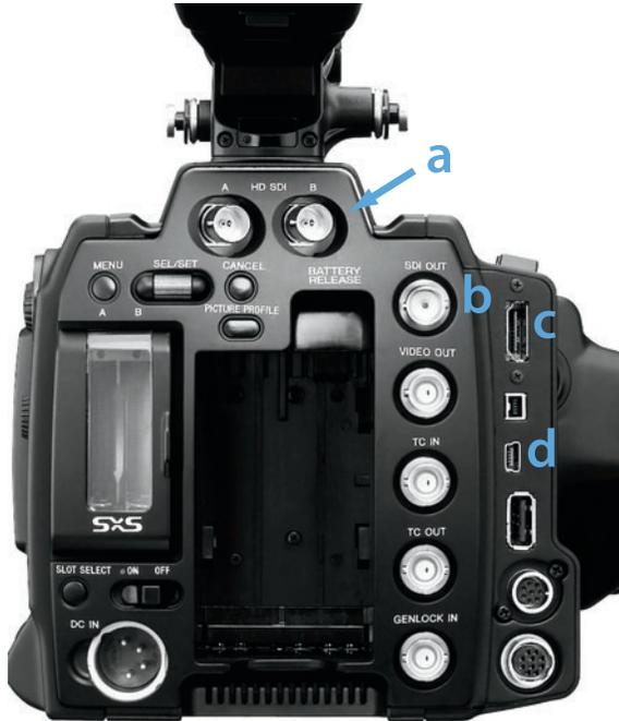
■ **Figure 9-11** Common video ports found on cameras usually include an HD-SDI (a) and SDI output and video output for monitoring (b), a HDMI port (c), and USB ports (d).
