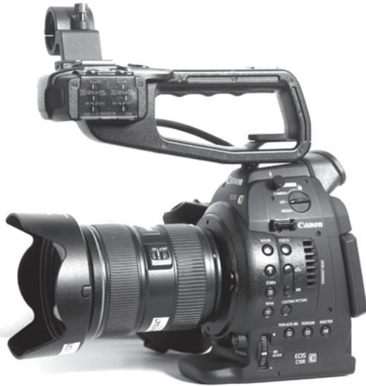
■ **Figure 9-33** Combining the best qualities of DSLRs (large sensor and interchangeable lenses) with the advantages of the camcorder (cinema prioritized functions), the hybrid camera, like this Canon C100, has become an extremely popular choice for high-quality, low-budget narrative film production.
