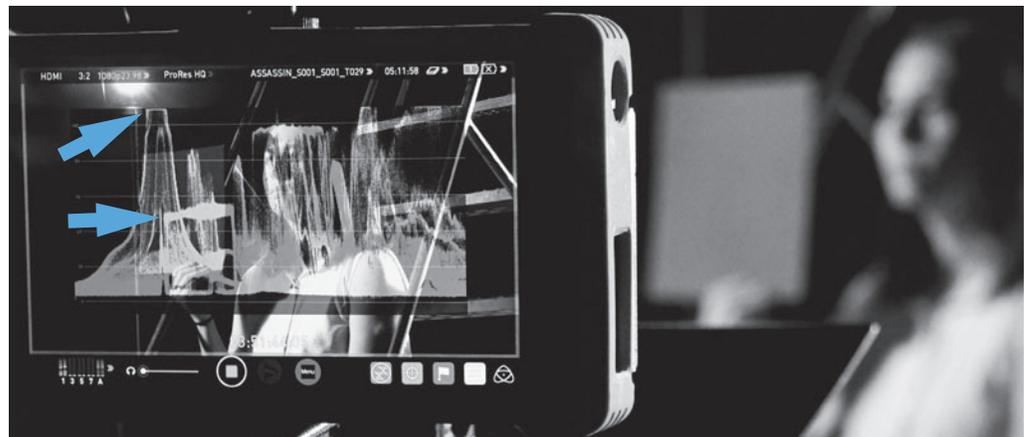
■ **Figure 14-17** The waveform monitor is an important exposure tool on a set. Many external field monitors come with a built-in WFM function, like this Atomos, that can display an image, or the waveform, or even overlay the waveform onto the image as seen here. Notice the bare light bulb clip above 100 IRE (*top arrow*) and the middle gray card expose at 50 IRE (*bottom arrow*).
