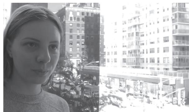
■ **Figure 13-35** Neutral density gels help control the extreme dynamic range caused by shooting against windows. This subject was shot in a relatively dark interior location with sunny streets visible through the window behind her. Taping ND9 gel on the window brings exterior and interior exposures closer (left half); the right half of the window was intentionally left uncovered.
