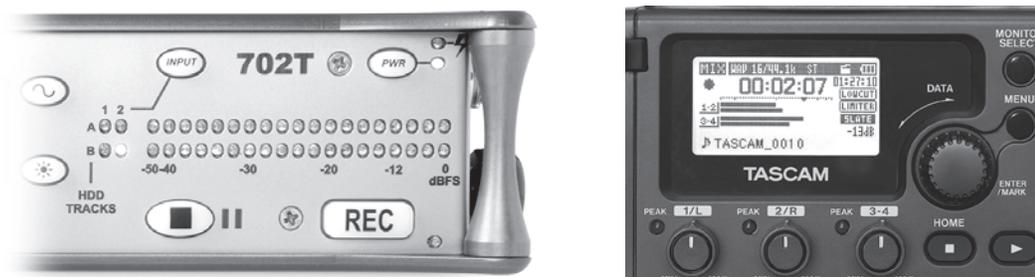
■ **Figure 15-18** Peak meters are essential for monitoring the strength of the signal being recorded. Peak meters can be LED based (left, showing a two-channel meter) and LCD based (right, showing a four-channel meter).
